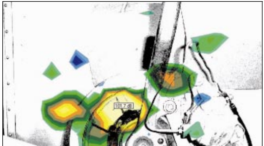
Fig. 1 Inside view of averaged narrow band intensity of a squealing brake. The contour plot is overlaid on a digital photograph of the brake
