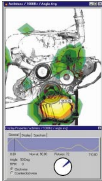
Fig. 3 Contour plot of a radiated sound field during engine run-up. The contour plot is overlaid on a digital photograph of the engine. Note the gauge for crank shaft angle. See also the front cover picture
